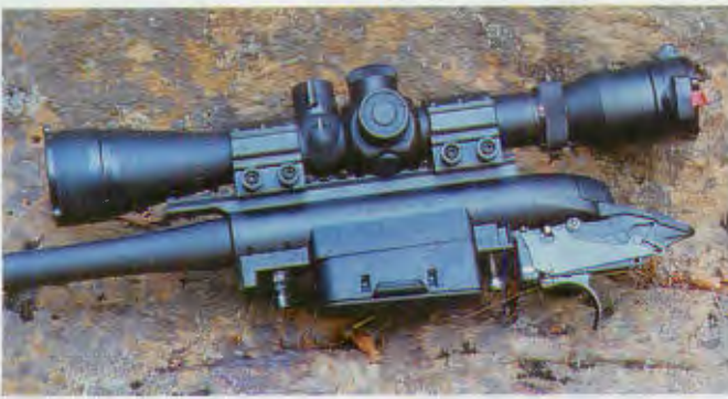
D.D. Ross machined the receiver and mounted his indestructible steel scope base. To this we mounted an I.O.R. tactical scope via D.D. Ross Extra H.D. Tactical rings. This is as bulletproof as it gets.
